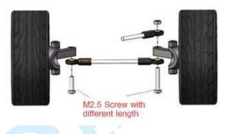
**No.5** Integrate No.3 and No.4 into the chassis, then fixed. Components List:
