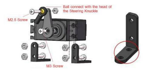
**No.4** Connect the Steering Knuckle – Connect the wheels of the No.2 with ball and rod, among that the hole space of the long rod is 65mm, else 48mm. Components List:
