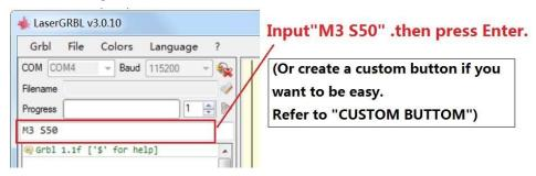
The laser will be turned on with low power model. Then Rotate the lens to minimize the spot.
