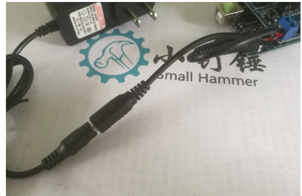
Figure Description: Detailed view of the DC barrel adapter conversion. Showing red wire matching '+' terminal and black wire matching '-' terminal leading safely to the V5 Shield power input.
