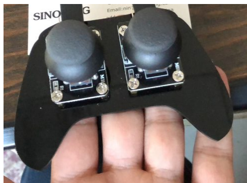
Figure Description: Top and angled view of the finished remote control handle, showcasing the twin joysticks securely screwed into place with thumb caps attached.
